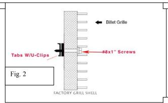
**Note**: Please adjust horizontal blades if irregular. This is the result of shipping and handling outside of Carriage Works control. Carriage Works recommends applying a high quality automotive wax to maintain the original appearance.
