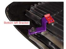
**STEP 5** Next attach the 2 outside angled Z-brackets (Left & Right side of Grille). Using U-clip and black #8 x 5/8 pan head screws. Then attach billet grille to stock shell using factory bolts as shown above.
