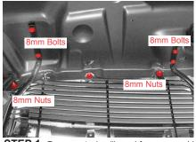
**STEP 1** Remove stock grille and frame assembly from truck by removing (6)-8mm screws holding frame. Remove (6)-8mm nuts from top edge of grille shell. As shown above.
