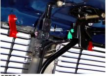
**STEP 8** Attach the 2 top Z-brackets using U-clips & black #8 x 5/8 pan head screw to attach to billet grille. Then using factory nuts attach to vehicle. NOTE: Before tightening all the bolts and nuts down be sure that the billet grille is centered in the opening. Once centered tighten all bolts & nuts.
