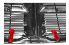
**STEP 7** Attach inside bottom left & right side Z-bracket to billet grille, using U-clips & black #8 x 5/8 pan head. Then attach brackets to stock grille shell using factory bolts. Re-attach grille assembl y.
