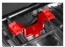
**STEP 6** Attach U-shaped bracket (Hat Bracket) to grille shell using U-clips & black #8 x 5/8 pan head screws. Shown above.
