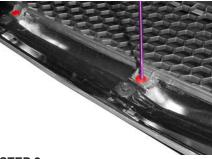
**STEP 2** After removing grille shell, lay grille face down on protective work surface (such as a blanket). Next punch center core (Qty 22) from plastic rivets holding grille inset in place, as shown above.
