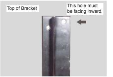
**STEP 2** Next you will be attaching the brackets for mounting the billet grille. Take note of the top hole in bracket this must point inward (Left bracket Shown).
