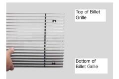
**STEP 4** Next you will be installing the billet grille. Take note that there is a top and bottom to the billet grille. The top (The tab is welded in the 3rd bar). The bottom (The tab is welded in the 2nd bar). Shown
