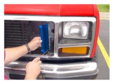
**STEP 3** Attach brackets to vehicle as shown (Bracket shown in Blue). Using factory clips & supplied #8 x 5/8" phillips pan head screws.
