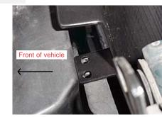
STEP 2 Then remove the mustang emblem. Align hood bracket and mark holes. Using a 9/32" drill marked locations. Then using the supplied 1/4-20 x 3/4" bolts and loc nuts attach the hood release bracket. NOTE: MAKE SURE BRACKET IS INSTALLED AS SHOWN. IF NOT PROPERLEY INSTALLED THE HOOD WILL NOT OPEN.
