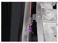
STEP 6 Mark location of bottom tab as shown above. Then remove billet grille and drill 1/8" hole at marked location.
