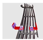
STEP 3 Attach Brackets loosely as shown above.
