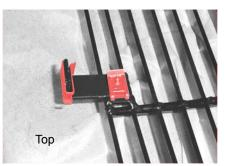
STEP 2 Attach upper and lower brackets using black #8 x 5/8" Phil. Pan Head screws and U-clips as shown. Then center grille between the headlights and against the bottom edge of the core support. Mark the location of the lower tabs and the center line of the top brackets.
