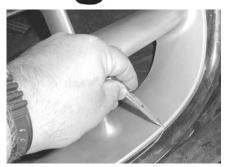
STEP 1 Remove grille shell. Cut center section of grille out along blend lines of grille shell as shown. Then sand contour of cut along blend lines. NOTE: IT IS VERY IMPORTANT TO SAND AS CLOSE AS POSSIBLE TO CONTOUR FOR IT IS A TIGHT FIT.
