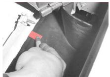
STEP 3 Drill an 1/8" hole in the lower marked positions.
