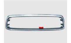
**STEP 2** Next cut out the center section of grille shell as shown above. DO NOT REMOVE CENTER BOSS ON BOTTOM OF SHELL MARKED IN RED. This is part of the hood release mechanism. Sand all raised bosses smooth. Repaint as needed.
