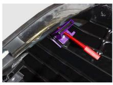
**STEP 5** Center billet grille in grille shell and mark locations of holes as shown above. Then drill a 1/8" hole for each.
