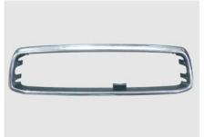
**STEP 1** Remove grille shell from truck and using masking tape to tape off the chrome or painted surface of the grille shell. To protect from scratching the face of the shell during install.
