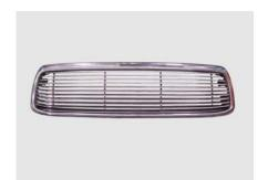
**STEP 6** Attach billet grille with remaining hardware and re-install the grille shell to truck.
