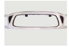
STEP 3 Using a cut-off wheel, cut center vertical sections out and sand smooth. If desired you may repaint sanded areas for a better appearance.
