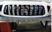
STEP 2 Tape off chrome or painted surfaces of grille shell. To protect face of grille shell.
