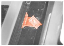
**STEP 3** Place U-Clips on bottom brackets of billet grille, center bilet grille then using factory screws to tighten.
