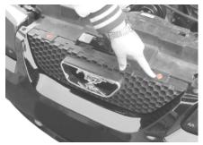
STEP 1 Remove 4 plastic rivets from top of grille shell
