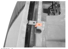
**STEP 5** Place the 2- U-Clips on core support using factory holes. Align grille bractets and use remaining 2 factory screws to tighten.
