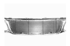
STEP 6 Now carefully place the billet grille into the back of grille shell. Center the grille in the opening. Mark the eight locations where the 1/4" rods meet the factory shell as shown above.
