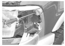
STEP 4 Remove the 2 screws behind parking lights
