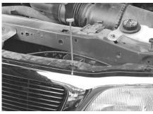
STEP 2 Then remove the 6 screws from the top of the grille shell.
