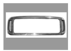
**STEP 3** Cut out the grey plastic center of the grille shell being careful to follow the small grey molded line described in step 2. After cutting the center out use a file to smooth out the edges. Again being careful to follow the grey molded line. NOTE: If installing center only skip step 4. You don't need to cut out the left and right pockets.
