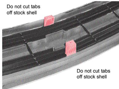
**STEP 2** Next cut the center sections of stock grille shell out. You need to leave the 2 center tabs shown in red above. Then file edges smooth with grille shell. See picture in step 1.
