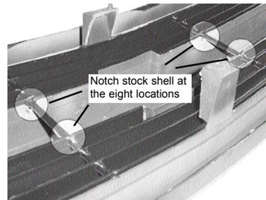
**STEP 3** Next knotch stock grille shell at the 8 locations shown above. Knotch 1/4" deep to allow billet grille to set flush with front of shell.
