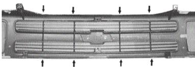
**STEP 4** Attach Billet Grille at the 8 locations with 1/8" pop rivets top & bottom of grille shell.
