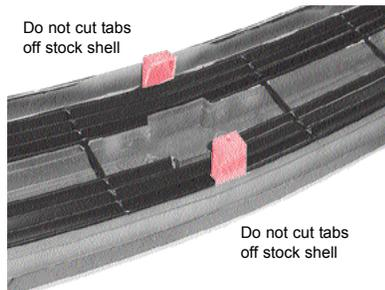
**STEP 2** Next cut the center sections of stock grille shell out. You need to leave the 2 center tabs shown in red above. Then file edges smooth with grille shell. See picture is step 1.
