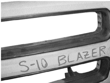
**STEP 1** Remove stock grille shell from vehicle. Then you can tape off the front of the shell using masking tape or by laying grille shell on a protective work surface such as a blanket to prevent any scratches to grille shell.
