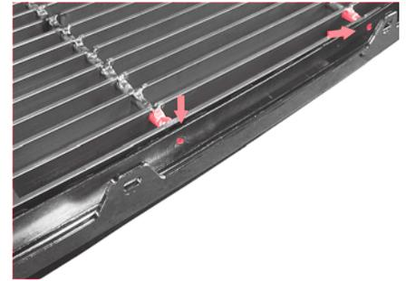
**STEP 1** Remove factory grille shell from vehicle. Then with some protective covering such as a blaket or rubber mat cover a work surface. So you don't scratch the front of your grille shell.
