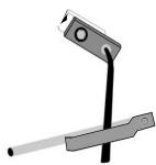
Step 6 (1999-2004) If your vehicle falls in these years skip step 5. Install the hood release by clamping the extension onto the hood release with the rod pointing downward and toward the front of the truck. Drill a  $\chi$ " hole thru the factory hood lever & attach with supplied bolts. Attach the long bracket using the factory hole in the tube frame so the rod is between the bracket and the tube frame and tighten the bracket in place.
