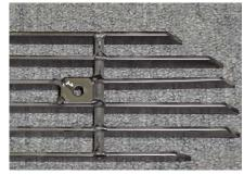
**Step 3** Looking at the Carriage Works billet grille, each individual grille will be stamped with a number on the back of the tabs. Placement will be as follows: 1-Driver side upper
