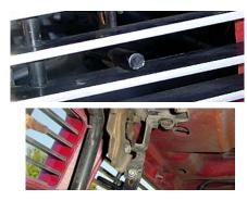
Step 5 (1997-1998) You will now need to install the hood release extension by clamping the extension onto the secondary hood release with the rod pointing toward the front. Mark and drill 1/4" holes and bolt in place. The extension will protrude just beyond the billet grille.(1997-1998) Remount factory shell with billet inserts onto truck. For 1999 & later see step 6.
