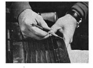
STEP 5 Loosely reinstall factory grill support and trial fit the new billet grilles into the factory shell. Tabs go to the top of shell; rods go to the bottom. Align billet inserts flush with the outer edges of grill support. With billet inserts in place, mark the four points on bottom of grille shell where vertical rods make contact. Drill 1/8" hole at center of each of these points.
