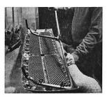
STEP 3 Lay grille, face down, on a stable work surface covered with a blanket or large towel. Finish removing the five 8 mm bolts on the metal grille support frame (loosened in step two).
