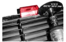
**STEP 4** Along the top of the grille shell there are 3 molded tabs (left,right,& center). Shown in red above. You will need to remove the center tab completely, using a cut-off wheel. Shown in red above.
