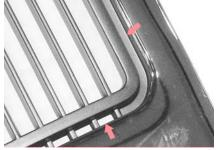
STEP 3 After removing center section grind or sand smooth all rough areas.
