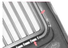
STEP 2 Remove the center section of grille shell by using a cut-off wheel. Cut along the outer most edge of grille shell as shown above.
