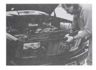
STEP 1 Remove parking lights. Then remove the grille shell.
