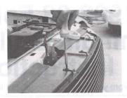
STEP 7 Mounting brackets on the top of the grille, attach in the original positions with the original mounting screws.
