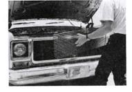
STEP 4 Take assembled grille to truck. Keep short grille bars and tapered ends of support brackets towards bottom of factory grille opening. Check alignment and fit.
