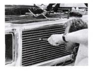
STEP 5 Once satisfied with alignment and fit, install new grille, using original 1/2" bolts. For starting bolts you will need a long extension, magnetic 1/2" socket or tape to hold bolt securely in the socket. Insert bolt, socket and extension through opening in the grille bars. It may be necessary to slightly spread bars to gain access to the mounting brackets. Tighten all 1/2" bolts and if needed, straighten grille bars in the new grille.
