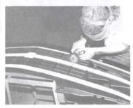
STEP 3 Cut the "egg crate" sections out of the grille. A cutting disc on an air-powered tool or electric drill works best, but a hack saw or saber saw will also do the trick. Be careful not to cut into the horizontal bars; the cuts will be dressed down cleanly later.
