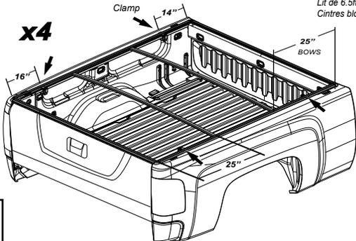
Align Clamp Assembly in the rail channel and begin to tighten the screw. Adjust all 4 Clamp Assemblies evenly. Tighten completely.
