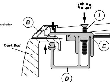
**NOTE:** When installing the clamps you may have to modify the bed-liner if present.
