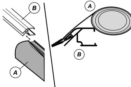
Slide into extrusion from end.
