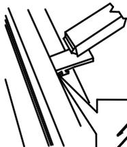
Insert bows to rail assembly by resting the bow on the top of the slider tabs with each of its legs draped over the sides. One bow is marked R for rear placement, the other bow is marked F for front placement on the truck rail assembly.
