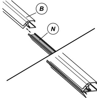
Insert tailgate seal "N" into the rear rail (marked with an "R") by sliding it in from the end.
