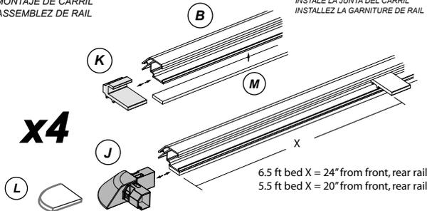
**Assemble rails by inserting Bow Slider into side rails, followed by an Endcap.**
