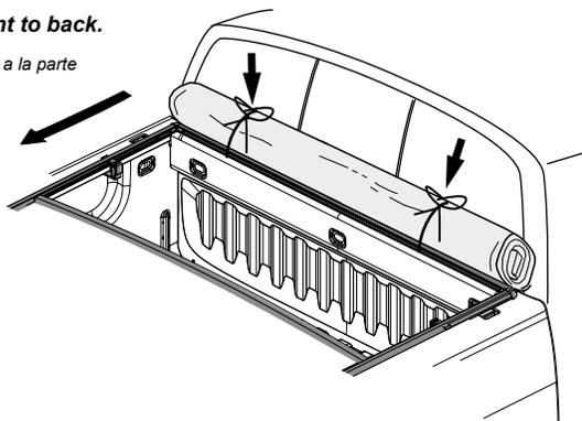
Starting at the front, tuck plastic retainer on the cover into the Rail Channel. Work towards the back of the vehicle.
