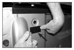
After short clamps are installed as shown on page 1, at rear of box under large hole in line with stake pocket, clean area and apply self adhesive protective strip.
