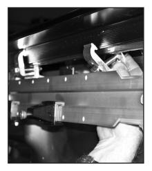
Do not disassemble clamp. Hold clamp as shown and reach up behind base rail. Then with clamp jaws open, tilt clamp and guide it to allow box lip to slip between clamp jaws.
