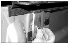
**4.** Place other half of clamp over bolt and turn nut on finger tight.
