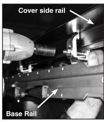
2. Hold clamp up as shown. Make sure clamp is located where two layers of sheet metal are present and tighten. Locate each clamp as shown on diagram and tighten.
