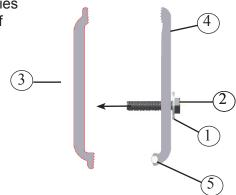
With TruXedo side rails in place, insert stake pocket clamp half into stake pocket. While holding stake pocket clamp half, insert male clamp half and bolt through the bolt hole of the stake pocket. Bolt clamp halfs together and tighten.
