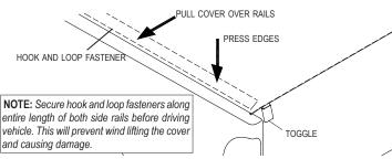
STEP 8: To release cover, Trigger pull rear release toggle. Start rolling cover toward cab making sure both sides of cover roll evenly. For best results leave unrolled portion of cover attached to the hook and loop fasteners while opening.
