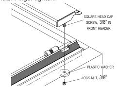
STEP 4: Set cover assembly behind cab with header seal on top of rail
