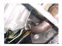
12) FINALLY, MAKE SURE ALL BOLTS ARE TIGHTEN AND EVERYTHING IS RECONNECTED. START THE ENGINE AND LET IT WARM UP. CHECK FOR LEAKS. TURN ENGINE OFF AND MAKE SURE ALL BOLTS ARE TIGHT. RETORQUE HEADERS AFTER 100-200 MILES.PERIODICALLY CHECK AND RETIGHTEN THE HEADER BOLTS. IF YOU DON'T RE-TORQUE YOUR HEADER BOLTS YOU COULD DEVELOP A LEAK AT THE HEAD GASKET. THIS IS NOT COVERED UNDER WARRANTY.
