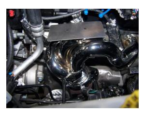
5. NOW ON PASSENGER SIDE REMOVE STOCK SHIELDS, SPARK PLUG WIRES, AND MANIFOLD. MAKE SURE TO CLEAN HEAD SURFACE OF ANY DEBRIS.
