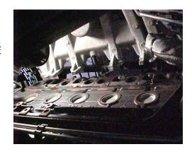
6. INSTALL GIBSON HEADER WITH SUPPLIED GASKET. AFTER HEADER IS BOLTED UP ON BOTH ENDS OF HEAD. INSTALL INTAKE MANIFOLD BACK ON, TORQUING ALL FASTENERS TO 35 - 35 FTS.
