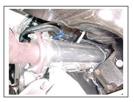
6. NOW CONNECT BATTERY CABLE BACK-UP AND CHECK FOR LEAKS. AFTER WARM UP LET ENGINE COOL DOWN AND TORQUE HEADERS ONE MORE TIME TO PREVENT LEAKS. THEN AFTER 200 TO 300 MILES RE-TORQUE HEADERS AGAIN. THEN WE RECOMMEND DOING THIS AT EVERY OIL CHANGE. THIS WILL ENSURE GIBSON HEADERS TO LAST TO THEIR FULLEST POTENTIAL.
