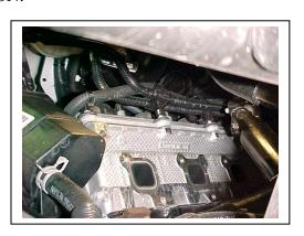
4. NOW NOTICE ON THE PASSENGER SIDE THAT YOUR TWO HEATER HOSES ARE CLOSE TO THE MANIFOLD. USE SUPPLIED Z-TIES TO TIE HEATER HOSES OUT OF THE WAY FROM THE LOG HEADER TO HELP PREVENT HEAT DAMAGE TO HOSES.
