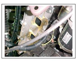
2. NOW ON DRIVERSIDE INSTALL GIBSON LOG HEADER AND SUPPLIED GASKET, HARDWARE TORQUEING TO 30 TO 35 FTLBS. AFTER LOG HEADER IS INSTALLED NOW INSTALL STARTER BACK INTO TRANSMISSION. NOW USING SUPPLIED HEADER-WRAP AND Z-TIES WRAP STARTER WIRES TO PROTECT THEM FROM ENGINE HEAT, AS SHOWN IN PICTURE!
