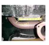
NOW STARTING ON PASS. SIDE FOR REMOVAL OF PASS. SIDE HEADPIPE. YOU WILL NEED TO MEASURE 3 ½" INCHES FROM CENTER OF BEND AND CUT WITH A HACKSAW OR SAWZALL SHOWN ON PICTURE. MAKE SURE TO DEBURR INSIDE OF REMAINING STOCK HEADPIPE.
