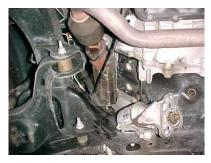
**4.** To remove the driver's side manifold. First remove the starter. Remove the driver's side manifold, stude and heat shields from the engine, through the top.
