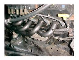
7. RE-INSTALL Y-PIPE WITH SUPPLIED HARDWARE AND TORQUE TO 30-35 FTS. CHECK ALL CONNECTIONS MAKING SURE THEY ARE ALL TIGHT. RE-INSTALL POSITIVE BATTERY CABLE.
