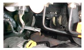
3. SPRAY WD-40 OR SOME TYPE OF PENETRATING OIL ON ALL ACCESSIBLE FASTENERS AND FITTINGS BEFORE ATTEMPTING TO REMOVE THEM.
