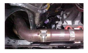
5. DISCONNECT ALL O2 SENSORS. THEN FROM UNDERNEATH THE VEHICLE, LOOSEN THE BOLTS CONNECTING THE Y-PIPE ASSEMBLY TO THE EXHAUST MANIFOLD. (ON 4X4 MODELS, DISCONNECT THE FRONT DRIVESHAFT BY REMOVING THE 4 BOLTS ON THE FLANGE, AND LET THE DRIVESHAFT HANG OUT OF THE WAY.)
