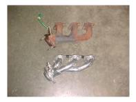
12.YOU CAN THEN INSTALL THE GIBSON HEADER USING SUPPLIED GASKETS AND HARDWARE. MAKE SURE TO USE ANTI-SIEZE ON HEADER BOLTS BEFORE INSTALLATION. TORQUE ALL HEADER BOLTS TO 30 FTS. THEN CONNECT EGR TUBE TO HEADER AND INSTALL SUPPLIED HEAT WRAP ON SPARK PLUG WIRES FOR BEST PROTECTION.
