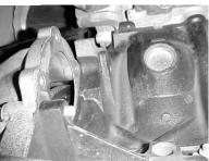
REMOVE THE MANIFOLDS ATTACHING STUDS.
