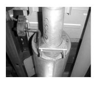
3. SLIP THE MUFFLER #B ONTO HEADPIPE #A NO LESS THEN 1- ½" AND NO MORE THEN 2". THE MUFFLER OUTLETS WILL BE LEVEL AT THE 12 O'CLOCK POSITION. THEN INSTALL HANGER #F ON THE INLET OF THE MUFFLER AND INSERT WELDED HANGER INTO RUBBER GROMMET. DO NOT TIGHTEN.
