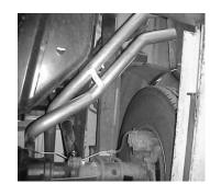
5.SLIP OVERAXLE PIPE #C ON THE PASSENGER SIDE OUTLET OF THE MUFFLER NO LESS THEN 1 1/2" AND NO MORE THEN 2". ATTACH TO MUFFLER USING CLAMP #G. DO NOT TIGHTEN. SLIP OVERAXLE PIPE #D INTO THE DRIVER SIDE MUFFLER **OUTLET AND ATTACH WITH** HANGER #J. NOTE: DRIVER SIDE **OVERAXLE TAILPIPE ROUTES UNDER PASSENGER SIDE** OVERAXLE PIPE, ENDING UP IN FRONT OF PASSENGER SIDE OVERAXLE. ATTACH BOLT ASSEMBLY #I. DO NOT TIGHTEN
