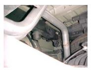
INSTALL DRIVERS SIDE TAILPIPE # D INTO MUFFLER 1 1 TO 2". INSERT WELDED HANGERS INTO RUBBER GROMMETS. USE CLAMP # H TO SECURE PIPE TO MUFFLER. DO NOT TIGHTEN.
