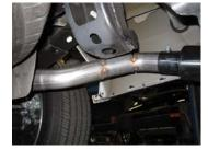
INSTALL EXIT PIPES # E & F ONTO TAILPIPES. ROTATE UNTIL LEVEL, USE CLAMP # H TO SECURE PIPES TOGETHER. DO NOT TIGHTEN.
