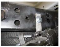
ON DRIVER SIDE: ATTACH REAR TAILPIPE HANGER #I TO FRAME USING BOLT KIT PROVIDED
