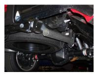
INSTALL EXIT PIPES # E ONTO TAILPIPES. ROTATE UNTIL LEVEL, USE CLAMP # H TO SECURE PIPES TOGETHER. DO NOT TIGHTEN.
