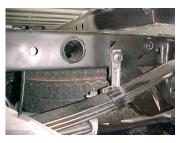
ON DRIVER SIDE: ATTACH REAR TAILPIPE HANGER #I TO FRAME BY REMOVING THE 18MM HITCH BOLT. THEN RE INSTALL BOLT WITH HANGER (IF YOU DO NOT HAVE A FACTORYHITCH USE BOLT KIT #L TO ATTACH HANGER #I TO THE FRAME RAIL. REPEAT ON PASSENGER SIDE.
