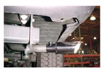
Install exit pipes # E onto tailpipes, and rotate until level.
