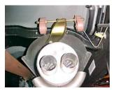
Install muffler #B onto head pipe  $1\frac{1}{2}$ " to 2" with the louvers facing towards the converter. Use a jack stand to support the muffler. Use clamp # H to secure the muffler to the head pipe. Do not tighten. Outlets should be on the bottom.
