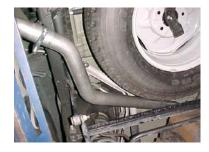
Next, install drivers side tailpipe # M into muffler 1-1/2" to 2" route between spare tire and shocks use clamp # G to secure do not tighten.
