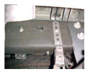
Measure approx. 12" from the rear of the frame and use the bolt that is there, and install 10" hanger # J use the 3<sup>rd</sup> hole on the hanger and install re-using the factory nut.
