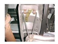
Next install both tailpipe hangers into rubber grommets. Then adjust it to your liking.
