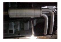
Install muffler assembly #A onto stock headpipe.
