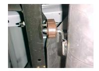
Install welded muffler hanger into rubber grommets.
