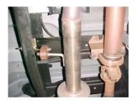
Install welded headpipe hanger into rubber grommet.
