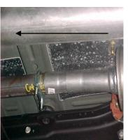
UNCLAMP STOCK MUFFLER. YOU WILL LEAVE THE FACTORY ALIGNMENT PIN IN PLACE. FOR EASIER REMOVAL HEAT UP CLAMP. CUT STOCK EXHUAST OFF AND USE WD-40 ON ALL HANGERS. LEAVE RUBBER GROMMETS IN PLACE.
