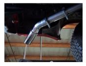
**8.** Next install the exit pipes #E. Use clamp #H, rotate pipes to the side. Trim ends of exitpipe to best fit your vehicle.
