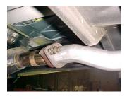
Slide flange # I onto your new head pipe #A then install head pipe #A onto you're existing stock flange using your factory hardware. Use a jack stand to support the converter.
