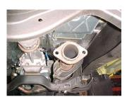
Lay out the exhaust on the floor so it looks like the drawing and compare parts with manual. To remove the stock exhaust remove it from the 2-bolt flange located in front of the muffler you will reuse your stock hardware. Leave all rubber grommets in place. Use WD-40 to aid in removal of exhaust and hangers. Use hacksaw to cut tailpipe off.
