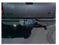
FINALLY AFTER TIGHTENING ALL CLAMPS FROM FRONT TO BACK AND MAKING SURE OF ALL CLEARENCES, INSTALL YOUR STAINLESS TIPS TO YOUR DESIRED LOOK.
