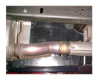
LAY OUT THE GIBSON EXHAUST ON THE FLOOR SO IT LOOKS LIKE THE DRAWING. COMPARE PART NUMBERS WITH MANUAL. TO REMOVE YOUR STOCK EXHAUST, REMOVE IT FROM THE CLAMP LOCATED JUST IN FRONT OF THE MUFFLER. YOU MAY NEED TO HEAT IT UP FOR EASIER REMOVAL. NOW CUT OFF YOUR STOCK TAILPIPE JUST BEHIND THE MUFFLER. USE WD-40 TO AID IN THE REMOVAL OF HANGERS. LEAVE ALL RUBBER GROMMETS IN PLACE.
