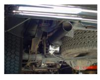
**INSTALL EXIT PIPES #F ONTO TAILPIPES,** ROTATE THE PIPE UNTIL IT IS AT THE PROPER LOOK FOR YOU. USE CLAMPS #I TO SECURE PIPES TOGETHER, DO NOT TIGHTEN.
