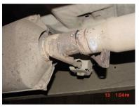
**TO REMOVE STOCK EXHAUST UNBOLT THE CLAMP LOCATED JUST BEHIND THE CATALYTIC CONVERTER.** FOR EASIER REMOVAL CUT THE STOCK TAILPIPE OFF JUST BEHIND THE MUFFLER AND REMOVE. LEAVE ALL RUBBER GROMMETS ON THE HANGER. USE WD-40 TO AID IN REMOVAL OF EXHAUST AND HANGERS.
