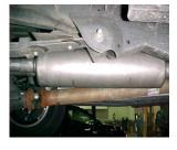
INSTALL MUFFLER # B ONTO HEADPIPE 1 ½" TO 2". USE CLAMP # F FO SECURE MUFFLER TO HEADPIPE. DO NOT TIGHTEN. USE A JACK STAND TO HOLD UP THE MUFFLER. DUTLETS SHOULD BE LEVEL.
