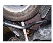
**6.** Install the driverside overaxle tailpipe #D into the muffler 1½-2". Use clamp #H to secure. DO NOT TIGHTEN. Rotate until it meets with the rubber grommet, use clamp #H to hold pipe. DO NOT TIGHTEN.
