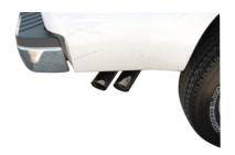
INSTALL YOUR STAINLESS TIPS. TIGHTEN ALL CLAMPS STARTING FROM THE FRONT, WORKING YOUR WAY TO THE BACK OF THE TRUCK. TO CLEAN TIPS USE A STAINLESS STEEL CLEANER & SCOTCH BTIE PAD.
