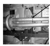
NEXT INSTALL HANGER # J TO DRIVERSIDE TAILPIPE AND INSERT WELDED HANGER INTO RUBBER GROMMET.MAKE SURE YOU HAVE EQUAL SPACE BETWEEN SHOCK AND SPARE TIRE. THE SPARE TIRE MAY NEED TO BE LOOSENED AND PUSH TO THE DRIVER SIDE AND THEN ROTATE THE OVERAXLE PIPE TO GAIN CLEARANCE.
