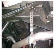
MAKE SURE YOU AT LEAST HAVE 1" CLEARANCE ON ALL BRAKE LINES, FUEL LINES, SHOCKS, TIRES, ETC.
